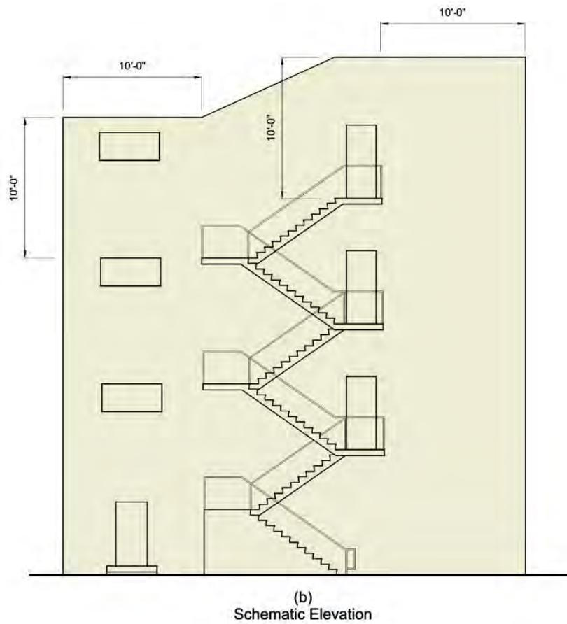
**SEPARATION AND PROTECTION OF EXTERIOR STAIRS**
