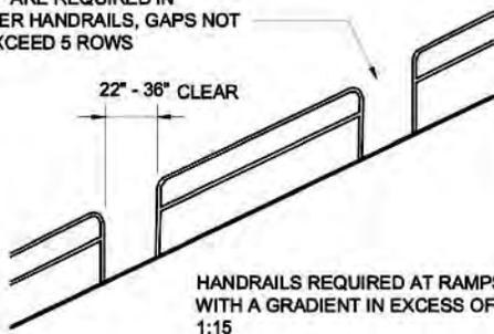
HANDRAILS REQUIRED AT RAMPS WITH A GRADIENT IN EXCESS OF 1:15
