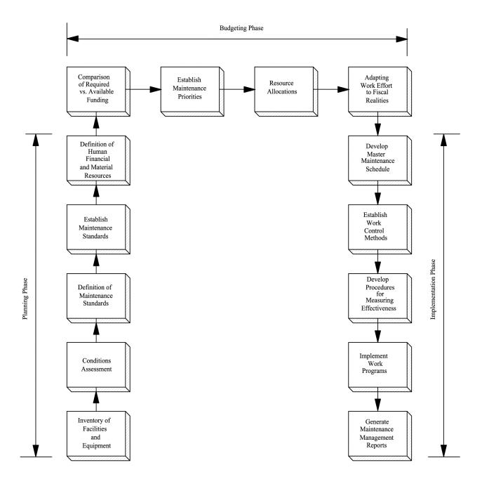
Figure 6.1: Flowchart for Implementing a Maintenance Management Program.
