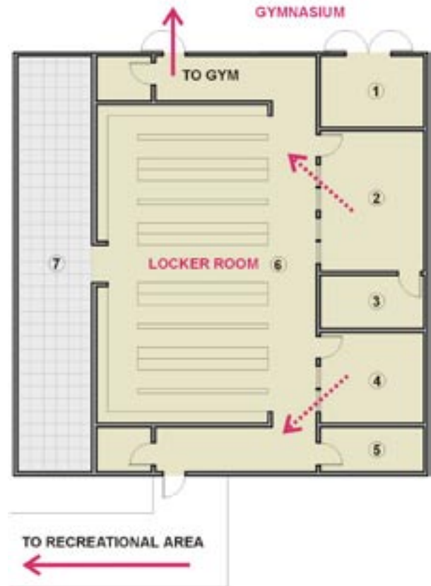
Figure 3.12.1 Plan Diagram Locker Room Schematic 1) Gymnasium Storage 2) Coach's Office 3) Coach's Toilet Room 4) Trainer's Office 5) Towel Storage 6) Changing Area and Lockers 7) Toilet and Shower Facilities
